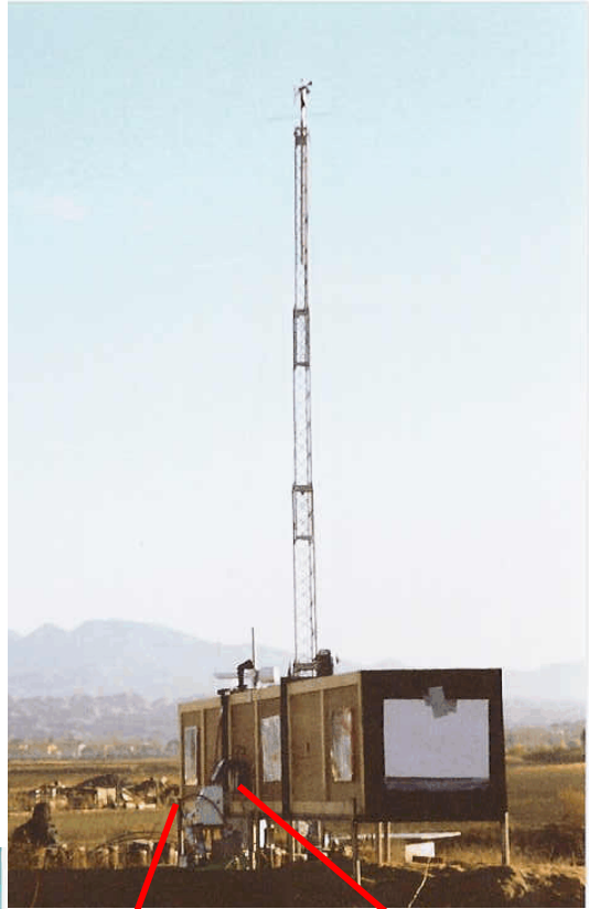
Figure 2. Chamber was used to generate and measure a controlled sample (clockwise views): (a) Front (west) and north sides of test chamber where samples are injected and measurements made, the chamber is shown with instrumented meteorological tower, (b) DustTrak optical scatter instruments (10 \mu\text{m} size orifice) and Climet particle spectrometer (16 channels - 0.5 to 10 \mu\text{m} ), (c) View of lidar from back of chamber at range of 450 meters thru the chamber (notice fans used to circulate the sample), (d) View of the east side of 10-meter chamber.
