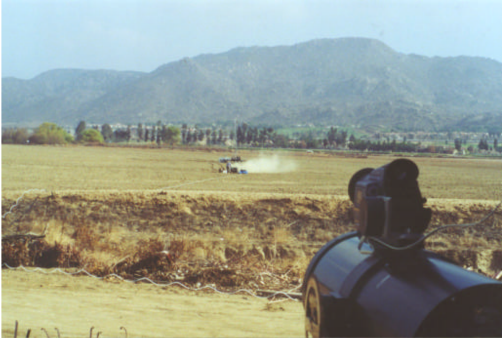
Figure 4.4. The lidar with a digital camera scans dust cloud generated by a blower, the 10 m tower is located directly behind the generator, and the target board can be seen in front of trees on the far left.
