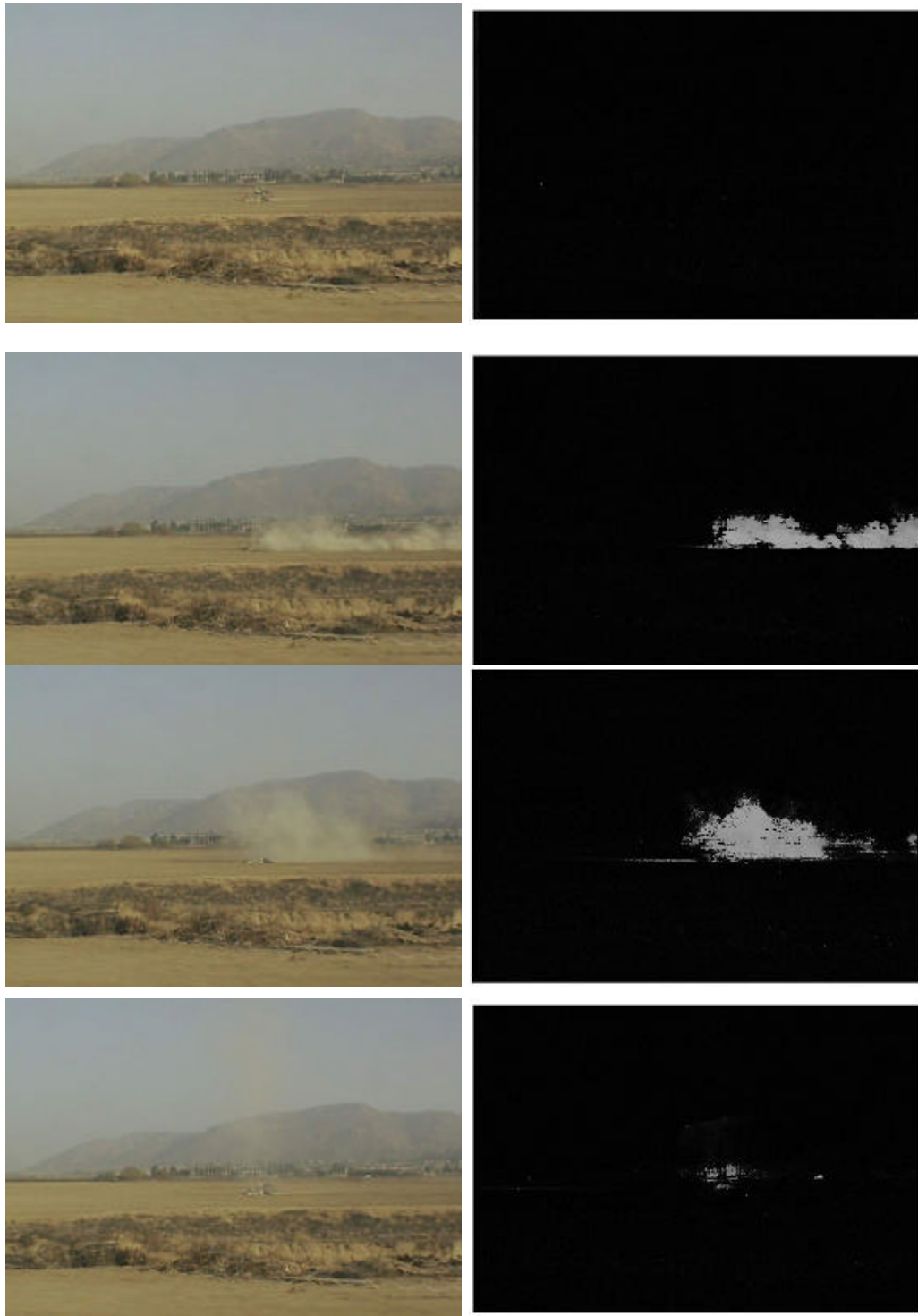
Figure 4.5. Test 18 (12/15/2000 14:30) generate dust with vehicle, this is time sequence of CCD images along with the corresponding background removed images: (a) 14:31:37 (b) 14:32:36 (c) 14:32:49 (d) 14:33:14.
