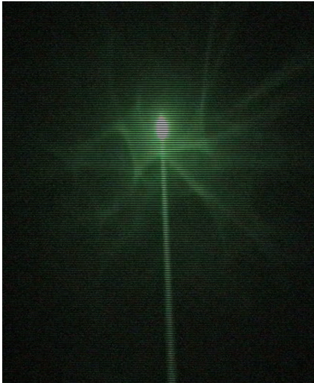
Figure 3.1. Second harmonic of the LAPS Nd:YAG laser scattering through a low cloud layer.
