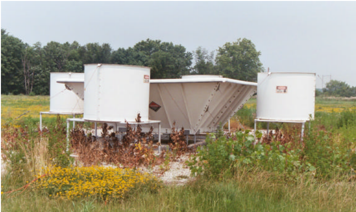
Figure 2.7 Wind profiling radar/RASS at the Philadelphia Baxter site (photo credit, C.R. Philbrick).
