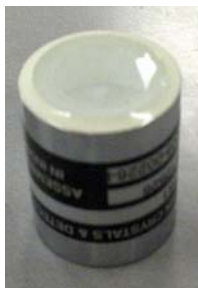
Figure 2.7: Packaged Sodium Iodide Crystal Used on HASP
