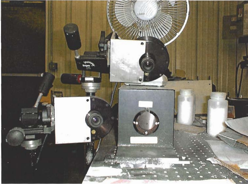
Figure 20: Two cameras, argon ion laser, and fan with cardboard box removed.
